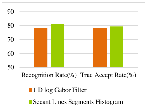
Figure 8. Comparison of Recognition Rate and True Accept Rate of 1D Log Gabor Filter and Secant Lines Segments Histogram
