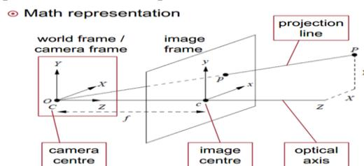
Figure2. Camera Calibration
