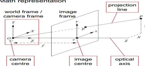
Figure2. Camera Calibration
