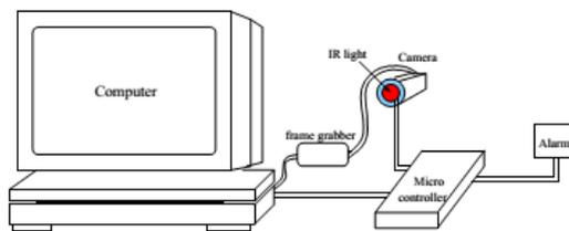
Figure 1. Typical hardware components of a computer vision system
