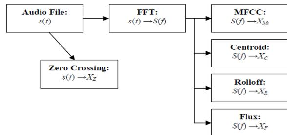
**Figure 3. Dataflow Diagram for Timbre Features**
