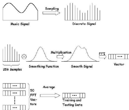
**Figure 2. Preprocessing of Audio Clip to Get the Input Data**
