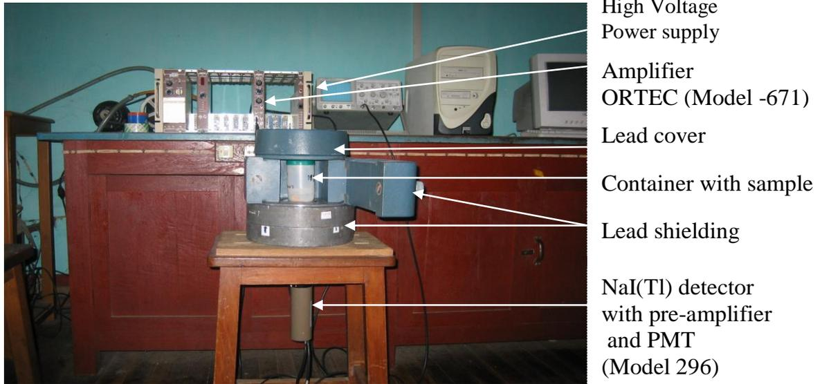
Fig.4.1 (a) Arrangement of experimental set up for detection system
