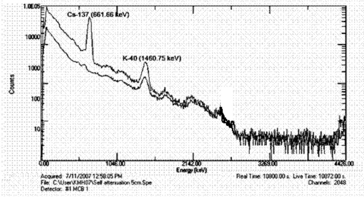
Fig.2 Comparison of Whey Powder sample and background spectrum.
