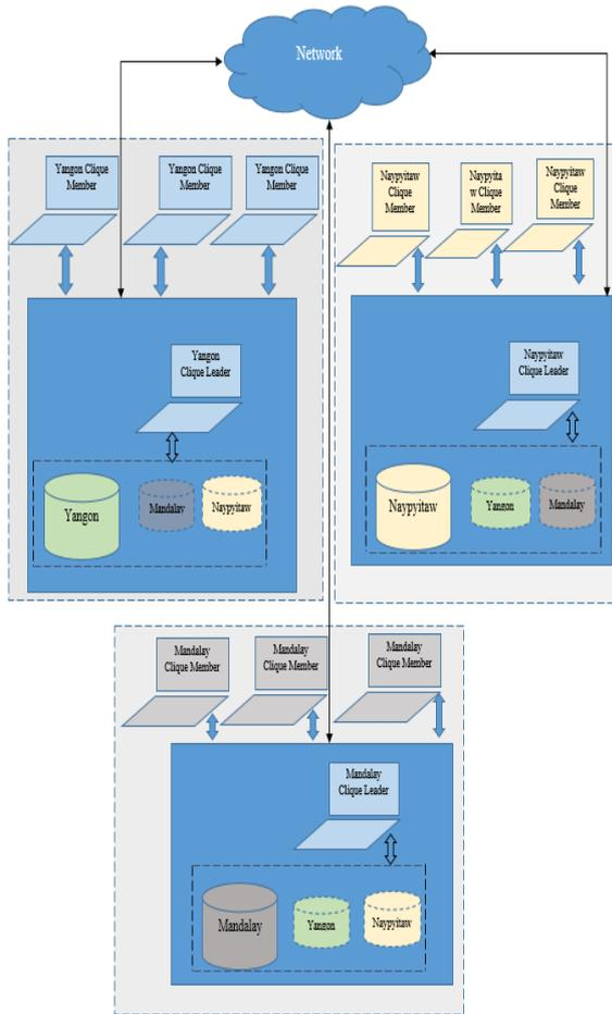
Figure 4. Station Diagram of Proposed System
