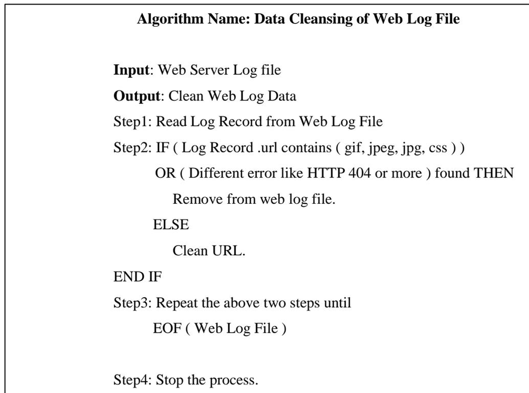
**Figure 4.1 Algorithm for Data Cleaning**
