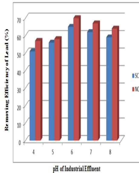
Figure (4) Effect of pH on Removal of Lead from Industrial Effluents by Treatment with Sulphonated Carbon
