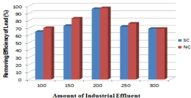
Figure (5) Effect of Amount of Sulphonated Carbon and Nitrated Carbon on Removal of Lead from Industrial Effluents
