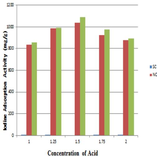
Figure (3) Effect of Concentrations of Sulphuric Acid and nitric acid on Iodine Adsorption Activity of Sulphonated Carbon (SC) and Nitrated Carbon (NC)
