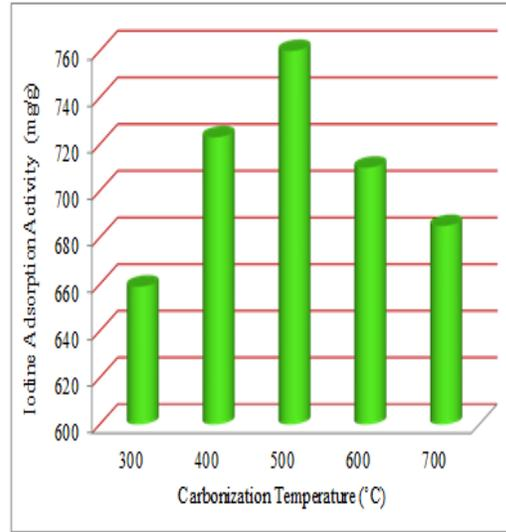
Figure (2) Effect of Carbonization Temperature on the Iodine Adsorption Activity of Carbonized Carbon
