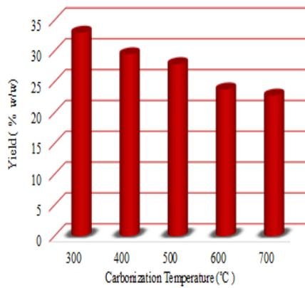
Figure (1) Effect of Carbonization Temperature on Yield Percent of Carbonized Carbon
