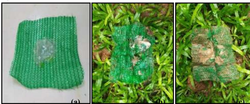
**Figure (1) Soil Burial Test for Biodegradable Plastic Film**
