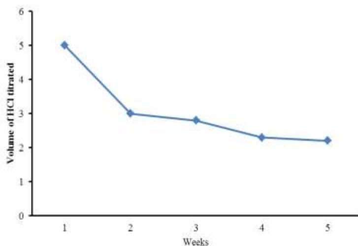
**Figure (3) Volume of HCl Needed to Titrate CO<sub>2</sub> Evolved from the Plastic Film**
