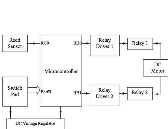
Figure 3. Block diagram of solar panel tracking section
