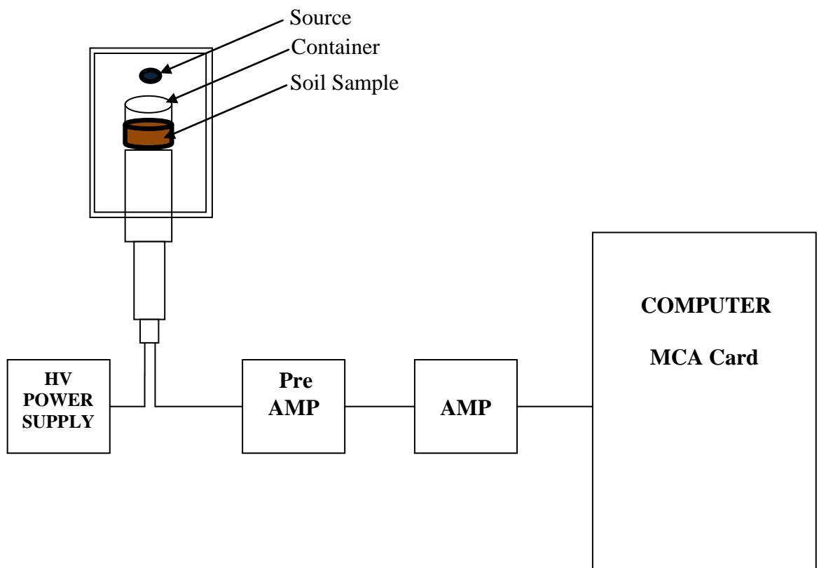
Fig. 3 Experimental Set-up of measuring system
