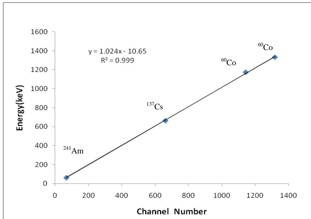
Fig. 1 Energy Calibration Curve
