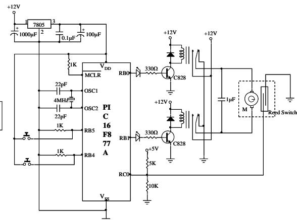
Figure 4. Complete circuit diagram of solar panel tracking section
