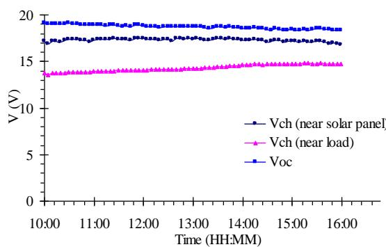
Figure 9. Voltage versus time graph without tracking
