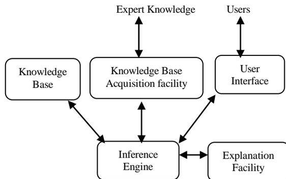
**Figure 1. Architecture of Expert System**
