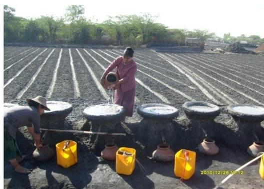
Figure (8) Filtering salt-water
