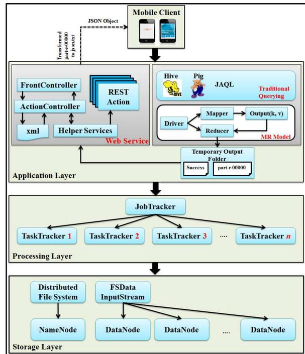
Figure 1. Mobile cloud platform architecture
