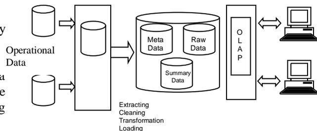
Figure.1 Architecture of a Data Warehouse with Staging Area
