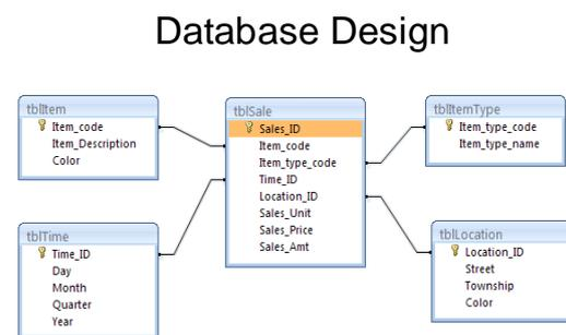
**Figure 2. Database Design (Star Schema)**
