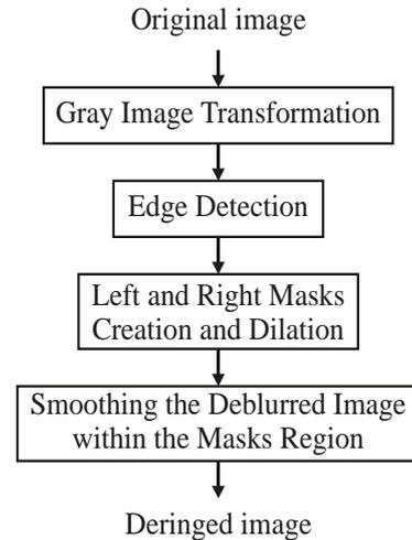
**Figure 8.** The block diagram representation of the deringing
