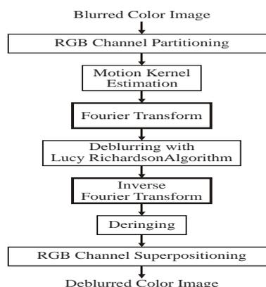
**Figure13.** Block diagram representation of the system
