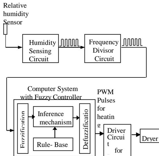
Figure 7. Block diagram of fuzzy logic dryer controller
