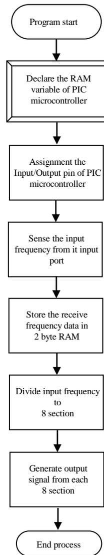
Figure 6. The flow chart of frequency sensing
