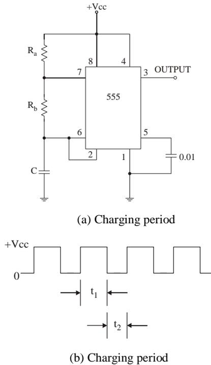
Figure 5. The 555 timer connected for astable operation
