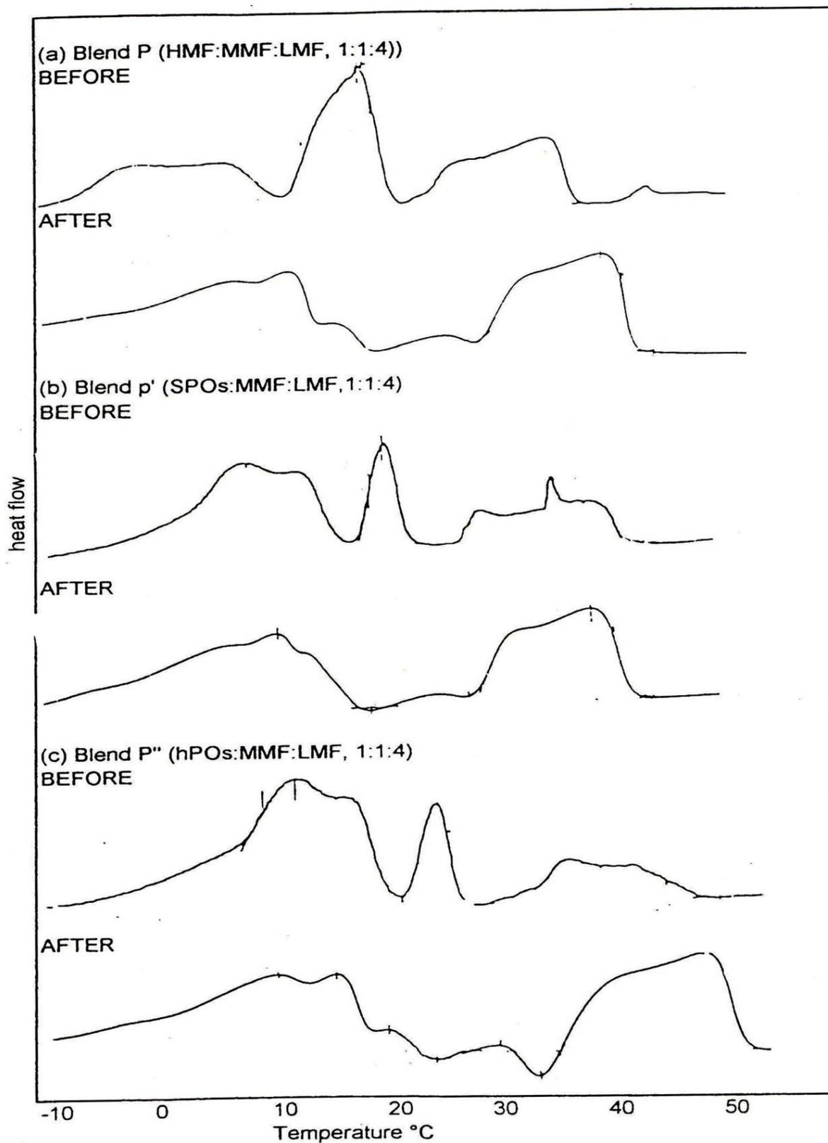
Figure 2 DSC melting profile of (a) HMF: MMF: LMF 1:1:4
