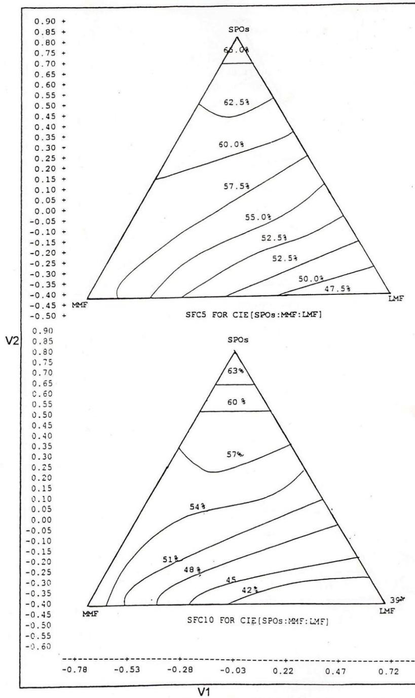
Figure 3c Iso-solid diagram of blends SPOs MMF:LMF at 5°C and 10°C before chemical interesterification
