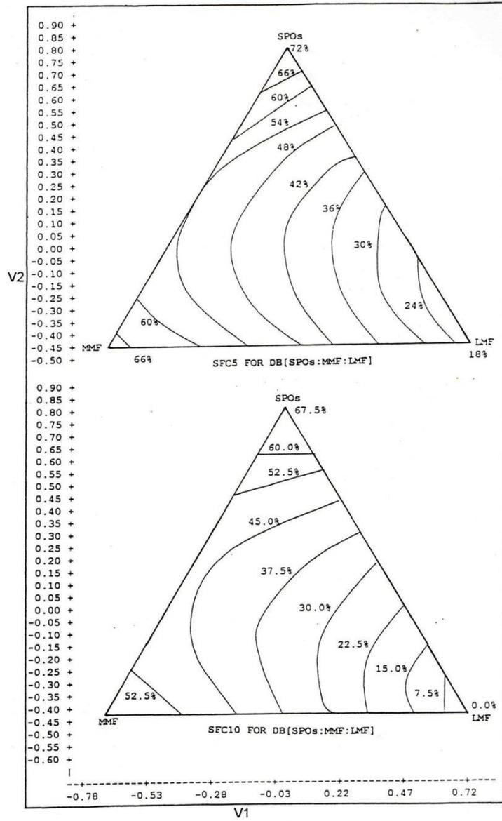
Figure 3a Iso-solid diagram of blends SPOs MMF:LMF at 5°C and 10°C before chemical interesterification
