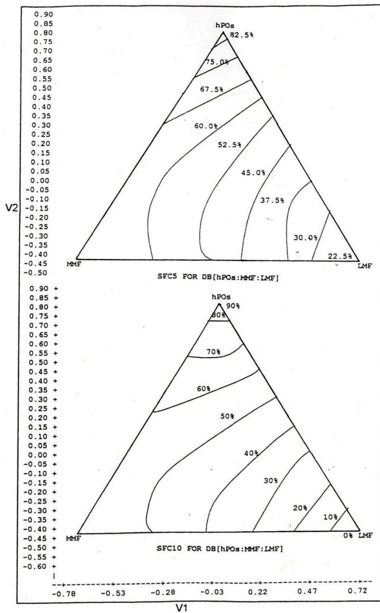
Figure 3b Iso-solid diagram of blends SPOs MMF:LMF at 5°C and 10°C before chemical interesterification
