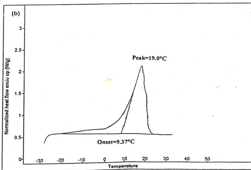
Figure 1b. DSC melting profile of (a) Commercial (b) laboratory MMF
