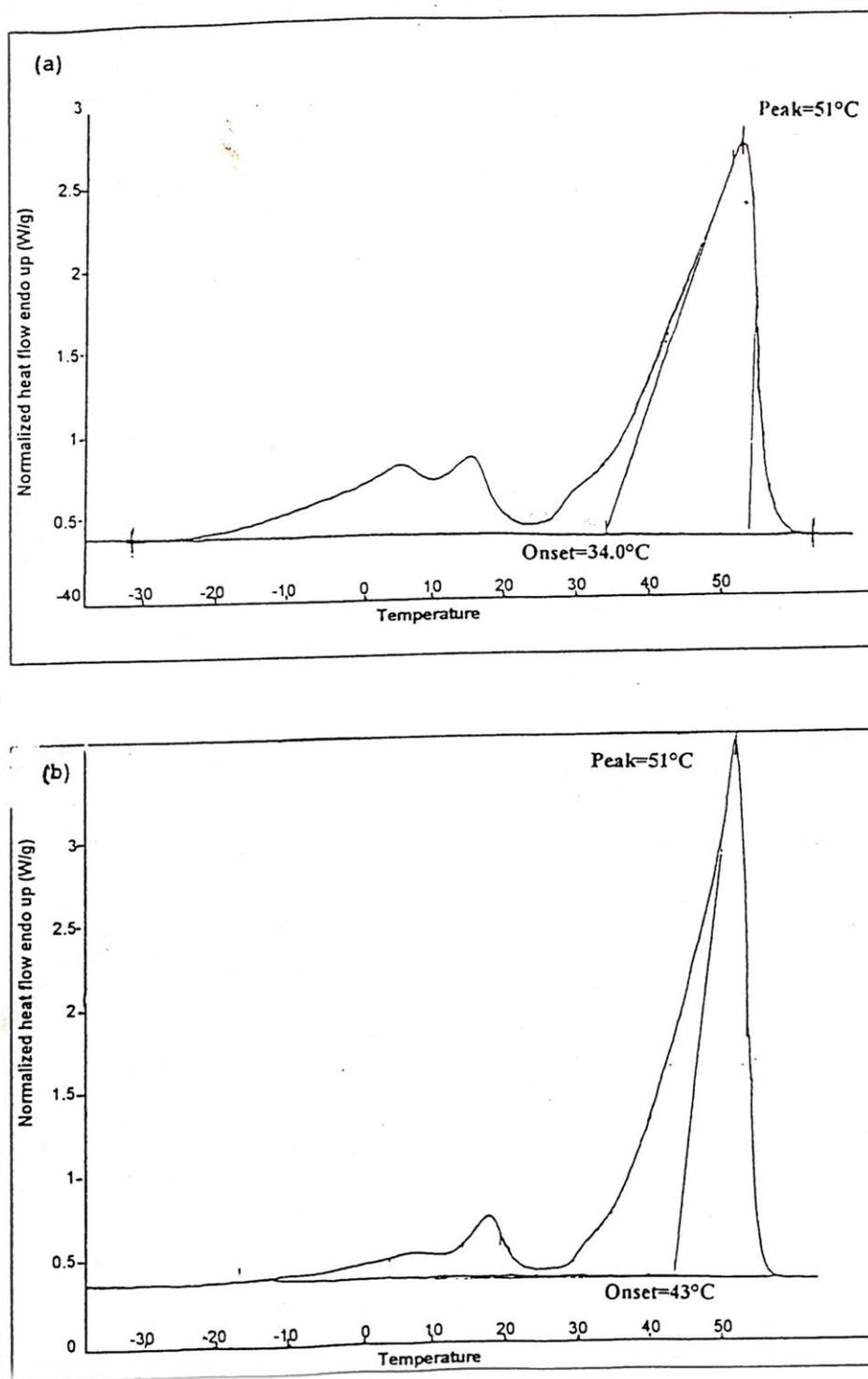
Figure 1.a DSC melting profile of (a) commercial (b) laboratory HMF
