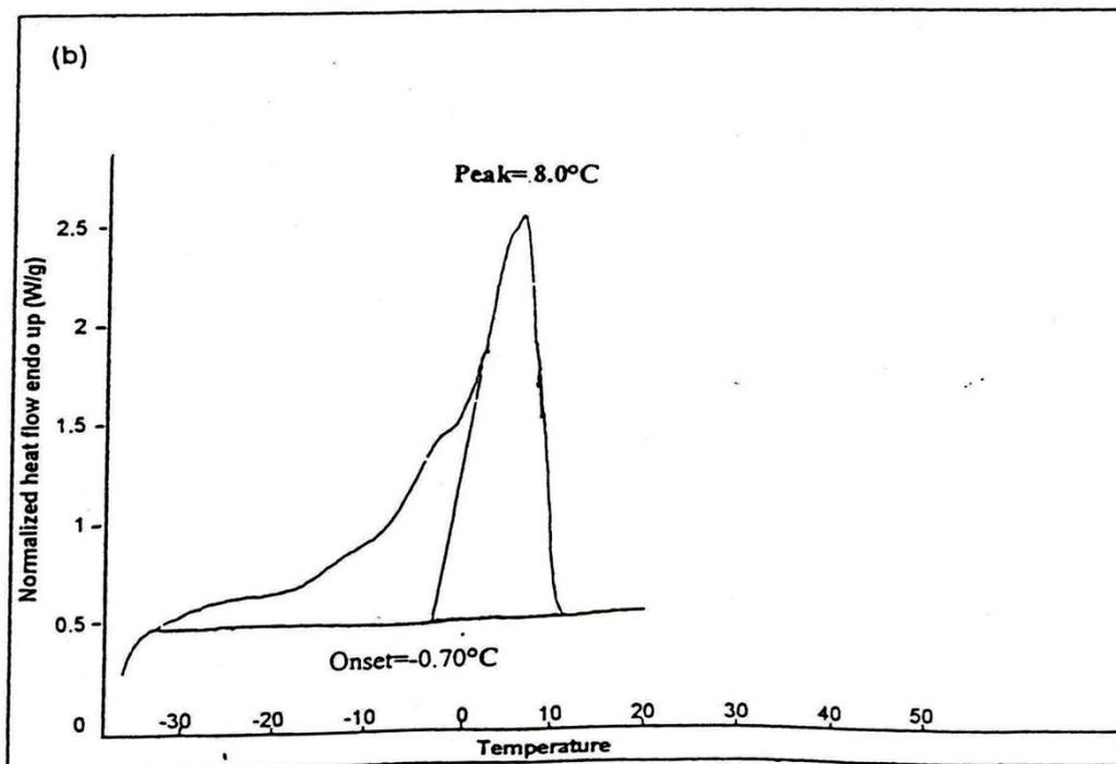
Figure 1c. DSC melting profile of (a) Commercial (b) laboratory LMF
