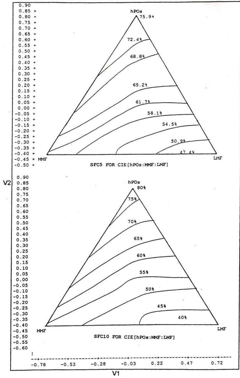
Figure 3d Iso-solid diagram of blends hPOs: MMF:LMF at 5°C and 10°C after chemical interesterification
