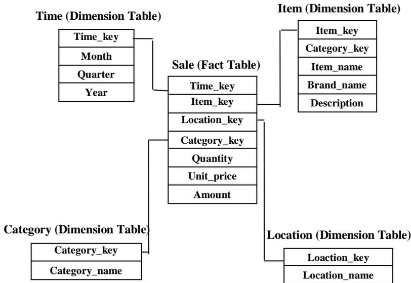
**Figure 4. Star Schema for Data Warehouse**
