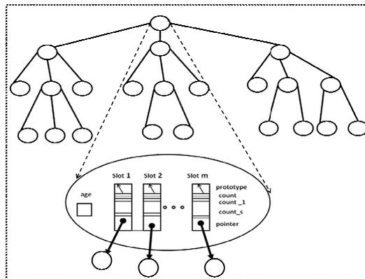
Figure.15. Tree structure of CNeT and node detail
