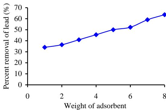
Figure 3. The Percent Removal of Lead from Lead (II) Nitrate Solution by Acid Treated Rice Husk Powder (by using Filtration Method)
