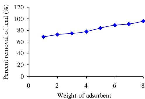
Figure 4. The Percent Removal of Lead from Lead (II) Nitrate Solution by Acid Treated Rice Husk Powder (by using Shaking Method)
