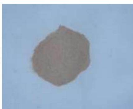
Figure 2. Tartaric Acid Treated Rice Husk Powder (60-80 mesh in size)
