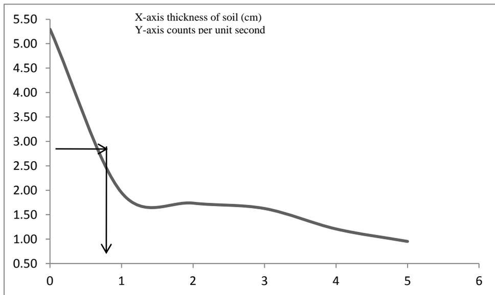
Fig. (2) Attenuation graph for Cs-137 Gamma Source (Ohn-chaw)
