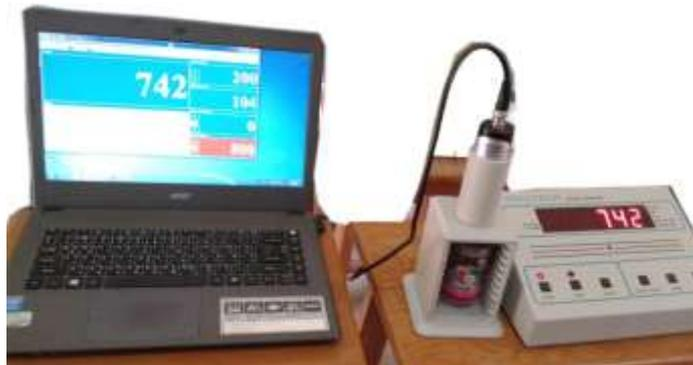
Fig. (3) The Photo of Gamma Ray Detection System
