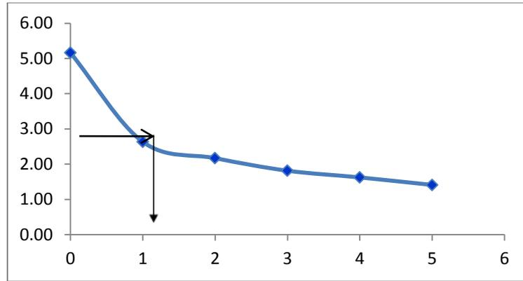
Fig. (4) Attenuation graph for Co-60 Gamma Source (Ohn-chaw)
