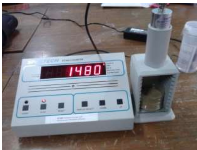
Figure 4. Experimental set up of GM counter
