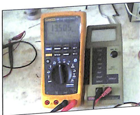
Figure 1 Fluke 289 Multimeter for measurements of resistance and conductivity
