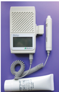
Figure 1. Handheld Doppler machine and transmission gel for detection of vascular flow (Bidop, model ES-100V3, Hadeco Inc., Japan)
