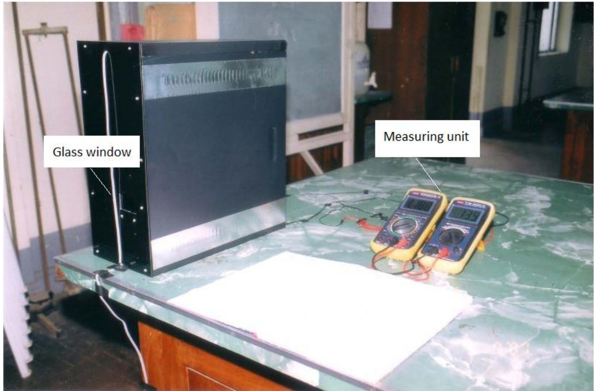
Fig 4.7 ( b ) External setup of photo-conductivity experiment
