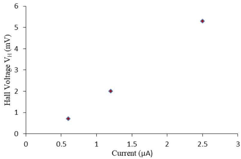
Fig 5.9 Variation of Hall voltages with current under the magnetic field of 500 mT
