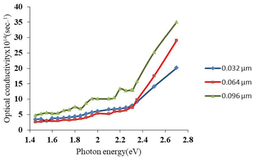
Fig 4.10 Optical conductivity ( $\sigma$ ) versus photon energy ( $h\nu$ ) of  $\text{Ag}_2\text{S}$  films
