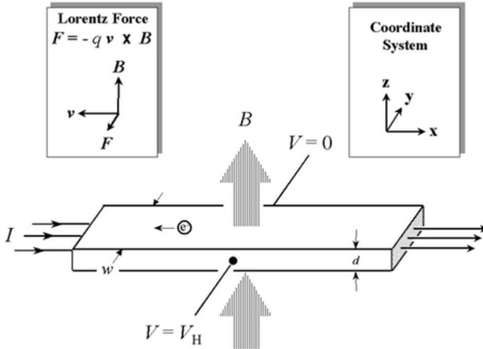
Fig 5.2 Schematic of the Hall effect in thin films with four ohmic contacts
