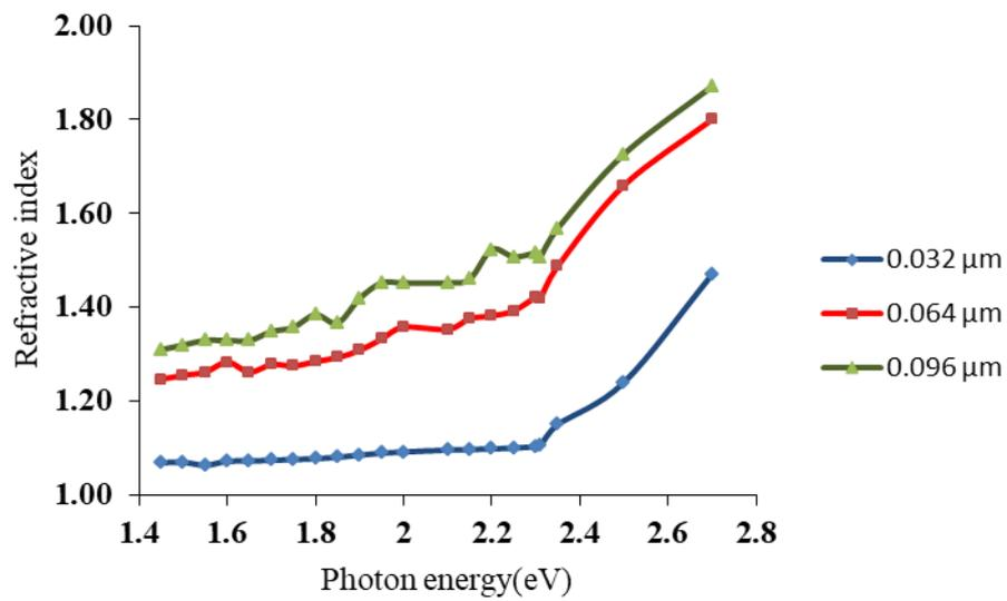
Fig 4.8 Refractive index ( $n$ ) versus photon energy ( $h\nu$ ) for  $\text{Ag}_2\text{S}$  thin films at different thickness
