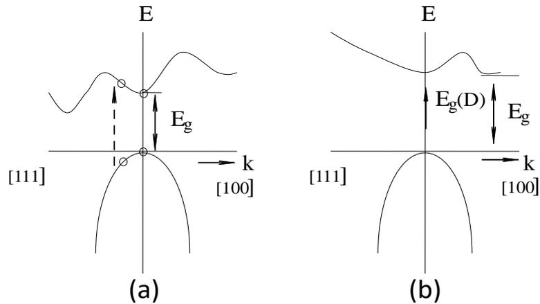
Fig 4.2 E-k plots for (a) Direct gap and (b) Indirect gap semiconductor
