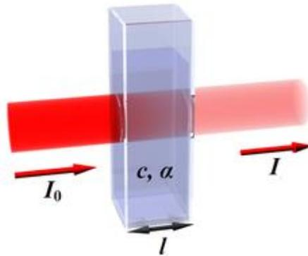
Fig 4.3 Diagram of Beer-Lambert Law of transmittance of a beam of light
