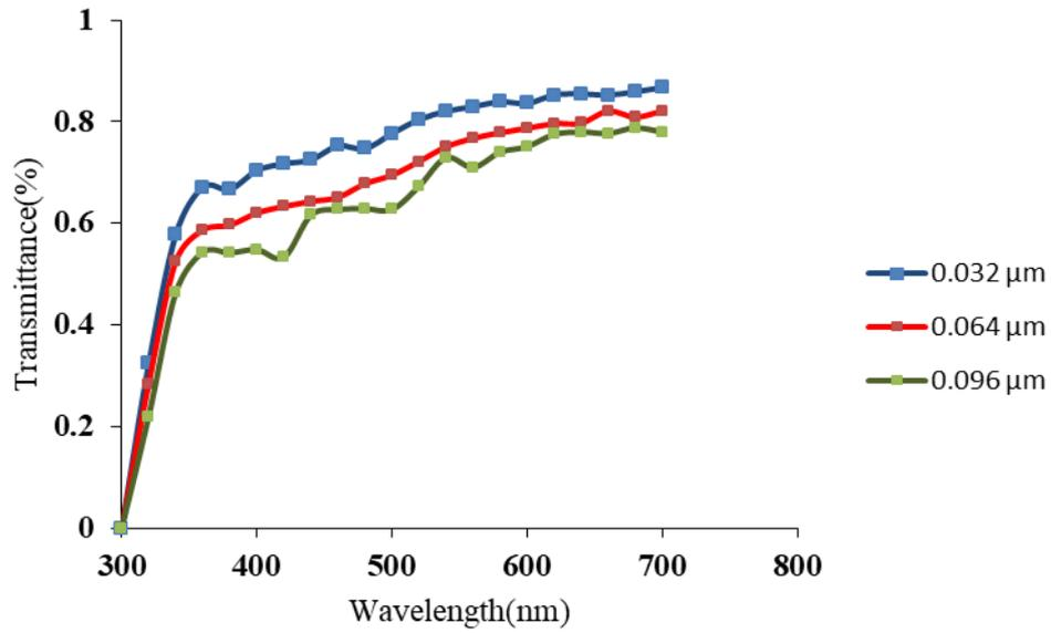
Fig 4.5 Optical transmittance spectra as a function of wavelength for thickness of  $\text{Ag}_2\text{S}$  film
