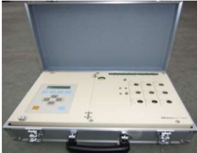
Figure 2: Instrument of Microtremor GPL- 6A3P Model, Mitutoyo Corporation.
