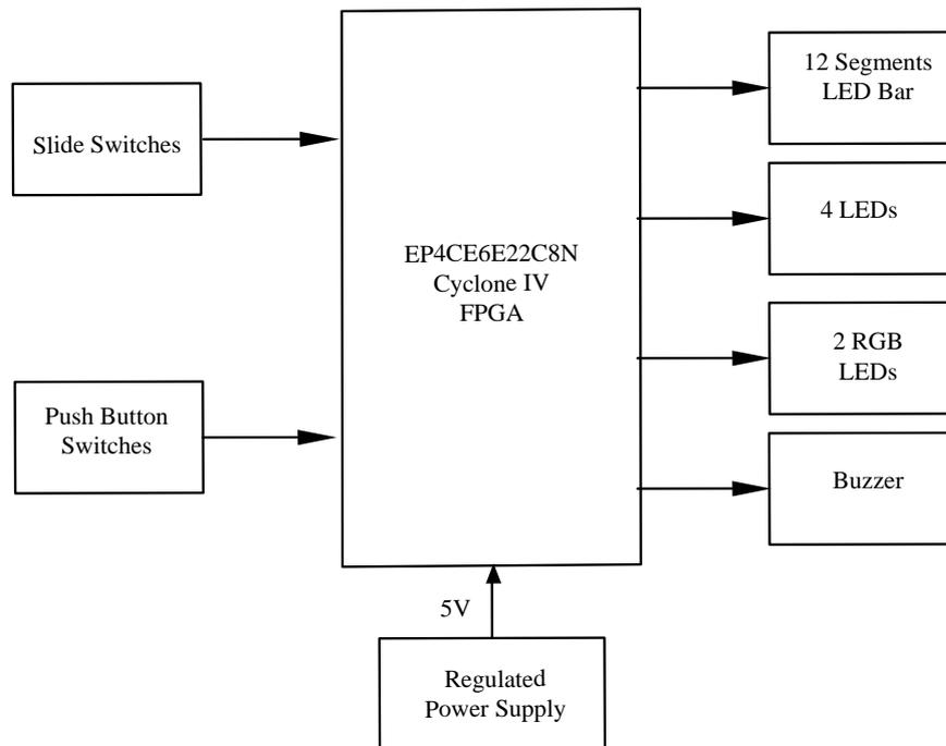
Fig.1 The functional block diagram of the constructed FPGA-based 3-digit 7-segments LED display counter
