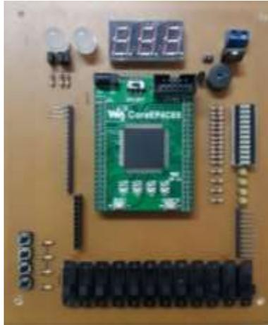
Fig.5 The photograph of FPGA core board and constructed circuit board.
