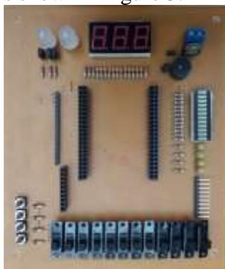
Fig.3 Constructed FPGA base board.
