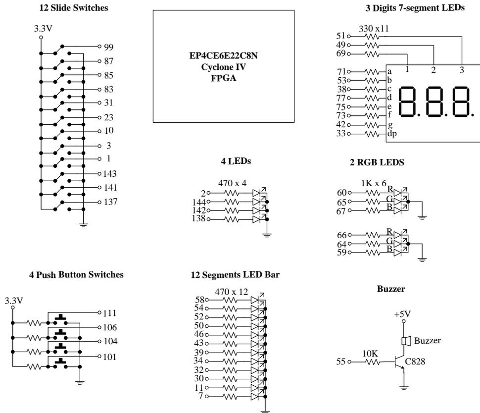
Fig.4 The complete circuit diagram
