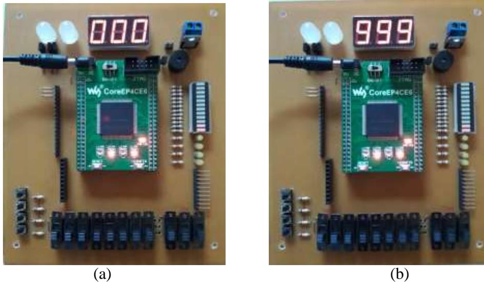
Fig. 7 The photographs of the constructed FPGA-based 3-digit 7-segments LED display counter (a) counting “000” and (b) counting “999”.
