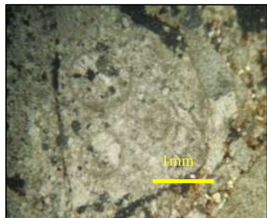
Fig. (22) Subrounded dolomitized biomicrite(a), dolomitized micrite(b) are cemented by silt matrix (XN)
