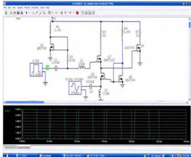
Fig. 6 Local oscillator input of simulated mixer
