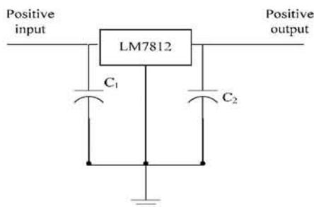
Fig. 4 Basic fixed-voltage regulator
