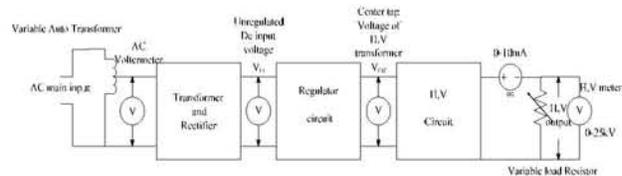
Fig. 6 A hook-up for measuring load and line regulation of H.V. Unit
