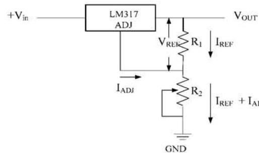
Fig. 5 Basic adjustable regulator using LM317IC
