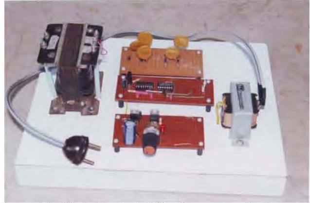
Fig. 7 Photo of constructed high voltage power supply unit
