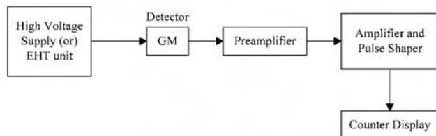
Fig. 2 Typical radiation detection system
