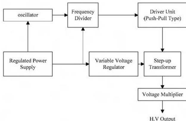
Fig. 1 Block diagram of high voltage unit
