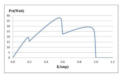
Figure 1. P-I curve of a string with 3 PV panels receiving 1000, 600 and 200W/m2 irradiations (left) and PV string with distributed DC/DC converter (right).
