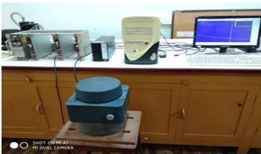
Figure 9. The detection system of NaI(Tl) detector
