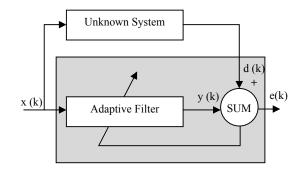
Fig. 3 Using an adaptive filter to identify an unknown system
