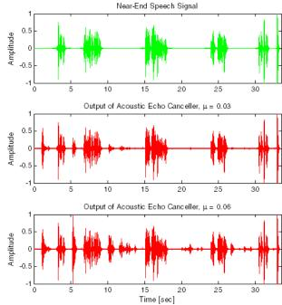
Fig. 8 Output of acoustic echo canceller with various step size
