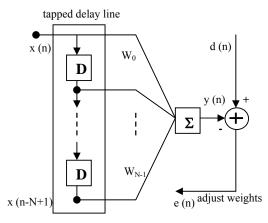
Fig. 4 Adaptive filter block diagram
