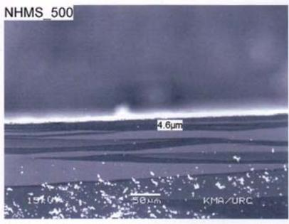
Fig 5 (c) SEM image of PCST film at 500 °C
