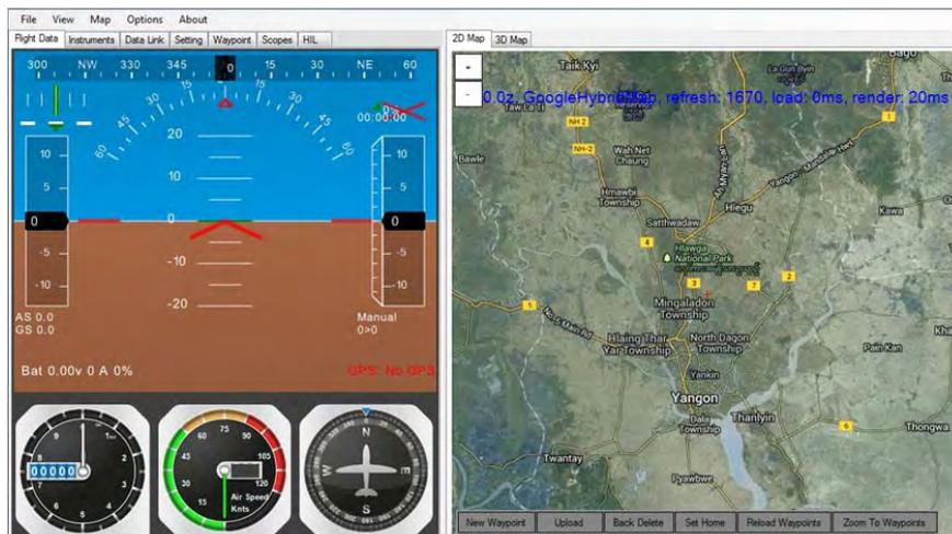
Fig.8 Ground Control System with Customized Map
