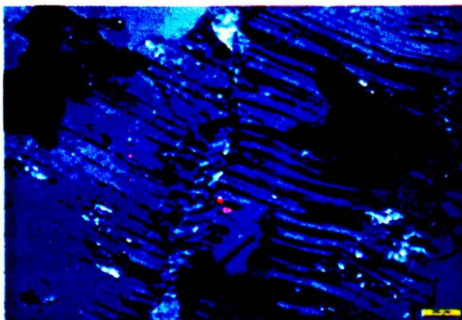
Fig. 12. Bending of feldspar with mineral inclusions (XN).
