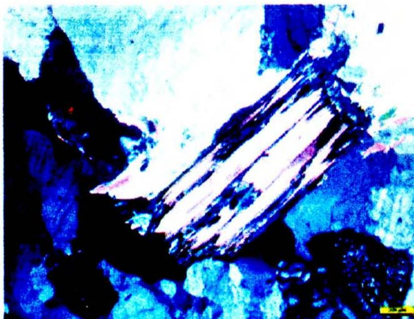
Fig.11. Chloritization of biotite and sericitization of feldspar in biotite granite.
