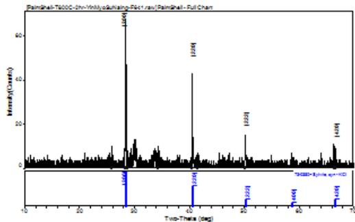
Fig.3(b). The XRD pattern of palm shell bio-char at 800 °C for 2h
