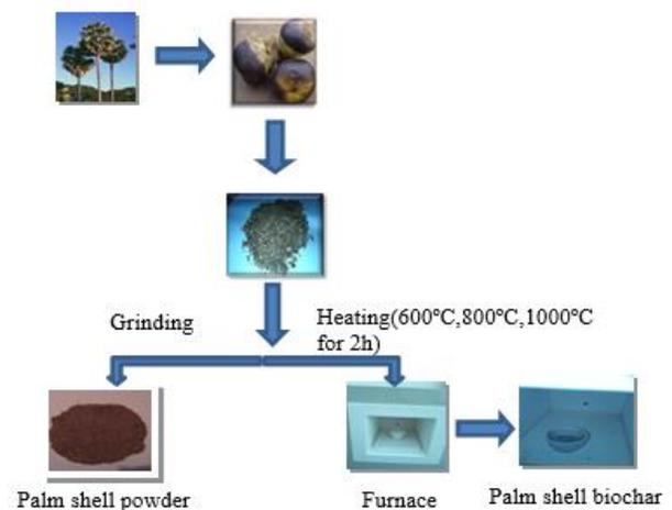
**Fig.1. Block diagram for experimental procedure of palm shell biochar.**
