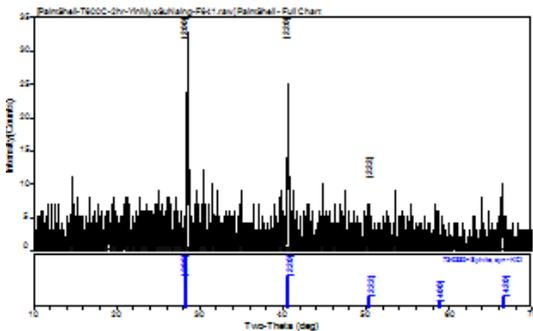
Fig.3(a). The XRD pattern of palm shell bio-char at 600 °C for 2h
