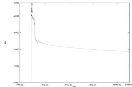
FIGURE. 3.(b) The optical absorption spectra of ZnO-SnO<sub>2</sub> nanocomposite film
