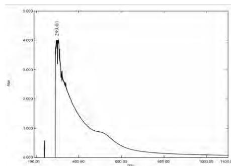
FIGURE. 3.(c) The optical absorption spectra of onion skin natural dye
