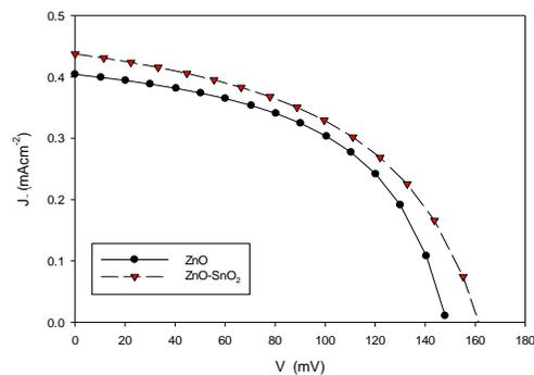
FIGURE. 4. J-V characteristic curve for ZnO and ZnO-SnO<sub>2</sub> nanocomposite electrode DSSC
