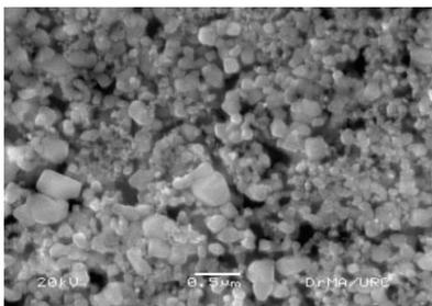
FIGURE 2.(b) Scanning electron image of ZnO-SnO<sub>2</sub> nanocomposite film
