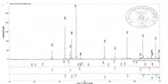
FIGURE 1.(b) XRD profile of ZnO-SnO<sub>2</sub> nanocomposite film
