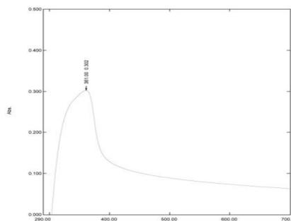
FIGURE 3.(a) The optical absorption spectra of ZnO nanorod film
