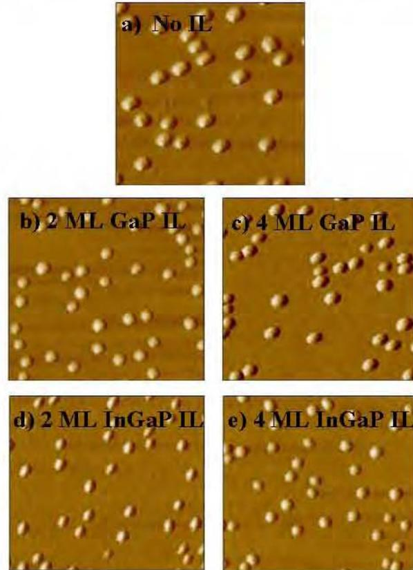
Fig. 2 Typical ( $1\mu\text{m} \times 1\mu\text{m}$ ) scan range AFM images of InP QDs embedded in InGaP barrier with GaP and InGaP insertion layers: (a) No IL (b) 2 ML GaP IL (c) 4 ML GaP IL (d) 2 ML InGaP IL (e) 4 ML InGaP IL
