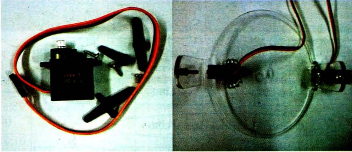
Figure 3. Tower Pro (MG90S) metal servo motor and insertion on the frame
