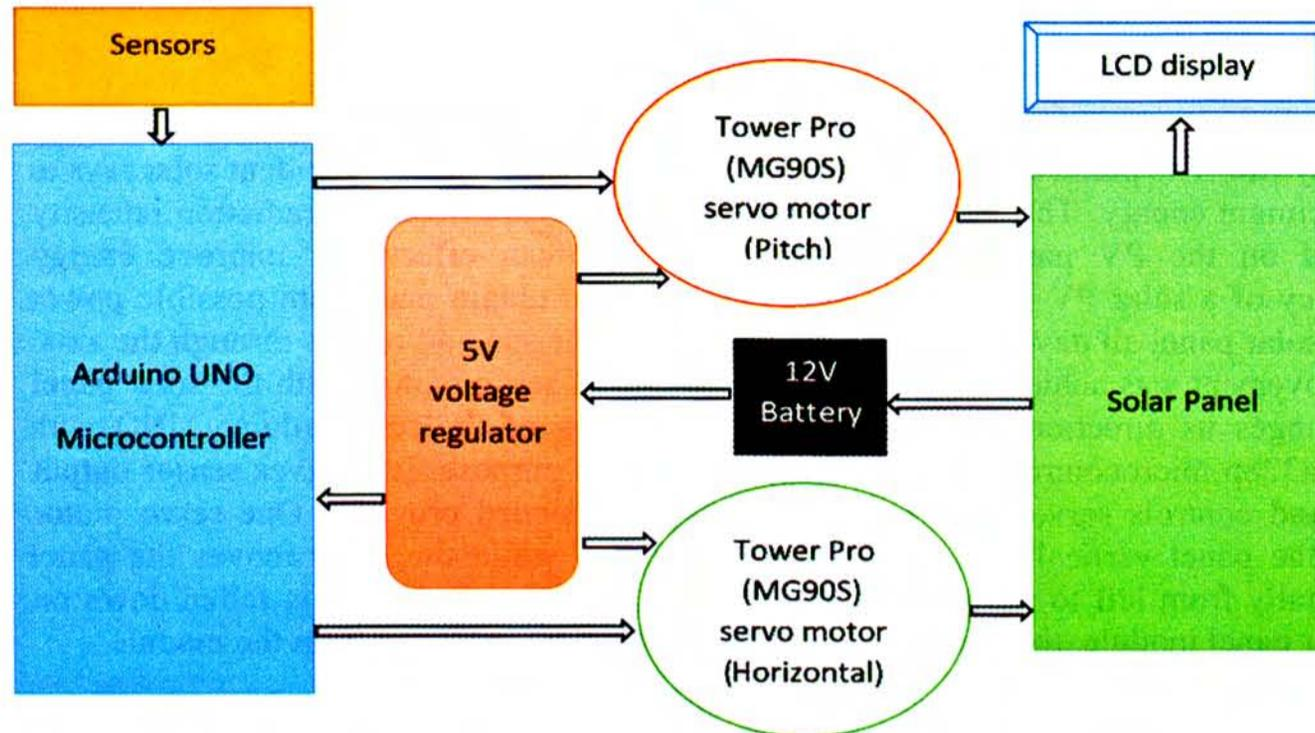
Figure 1. Block diagram of prototype dual axis solar tracker
