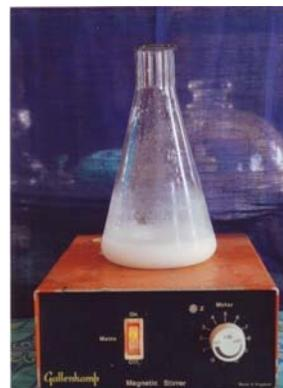
Figure 2 Magnetic stirrer with mixed solution
