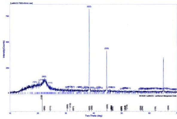
Fig. 6 XRD Patterns of LaMnO<sub>3</sub> fibres, annealing temperature at 800°C
