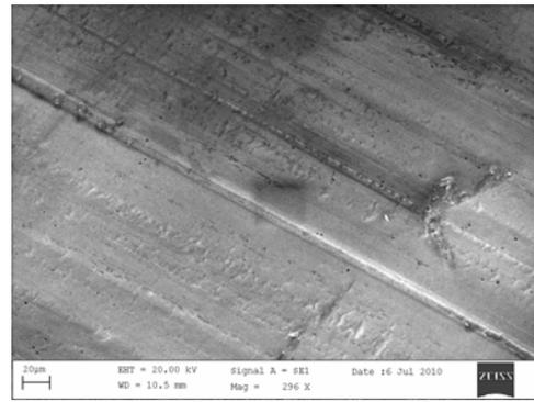
Fig. 7 (c) SEM image of lanthanum manganite La<sub>0.98</sub>Mn<sub>0.02</sub>O<sub>3</sub> fibre at 800°C
