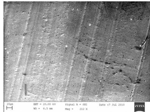
Fig. 7 (e) SEM image of lanthanum manganite La<sub>0.98</sub>Mn<sub>0.02</sub>O<sub>3</sub> fibre at 800°C
