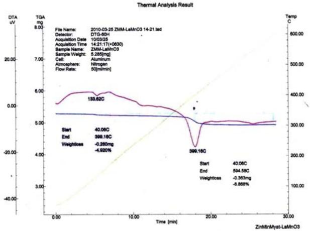
Fig. 3(c) TG-DTA analysis of La<sub>0.98</sub>Mn<sub>0.02</sub>O<sub>3</sub> powder
