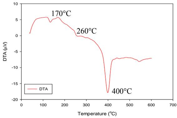
Fig. 3 (a) DTA analysis of La<sub>0.98</sub>Mn<sub>0.02</sub>O<sub>3</sub> powder
