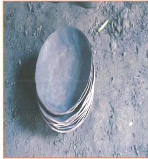
Figure-(4.60) Twelve layers are beaten together at a time
