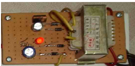
Fig. 11 Photo of constructed power supply
