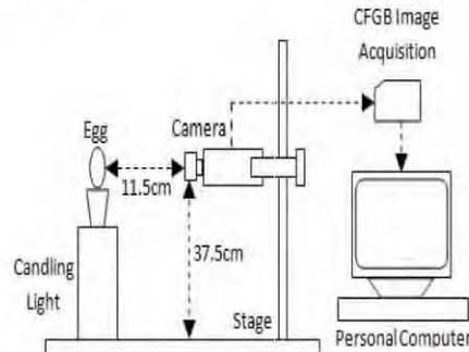
**Figure 1.** CV system for micro-crack detection of eggshell.
