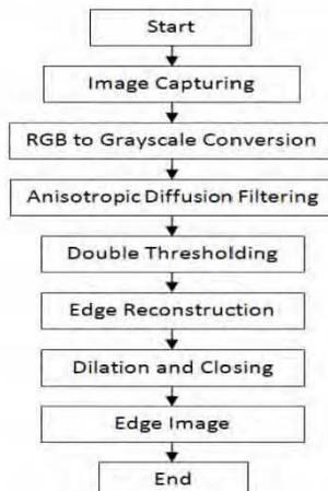
**Figure 4.** An algorithm for micro-crack detection of eggshell
