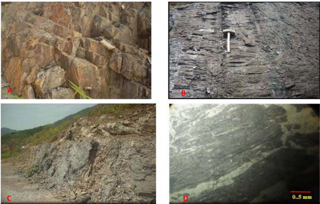
Figure.5 (A) Excellent exposure of phyllite at the eastern part of Kadaik Dam, Loc. N 050291, Facing 45° (B) Highly jointed nature of phyllite at the northeastern part of Zingyaik Taung (C) Slate intercalated with phyllite, at the eastern part of Zingyaik Taung, Loc. N038277, Facing -20° (D) Phyllitic texture in phyllite, Between X.
