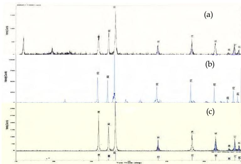
Fig. 1. XRD spectrum of (a)0.02M (b) 0.04M (c) 0.06M ZnO nanorod film
