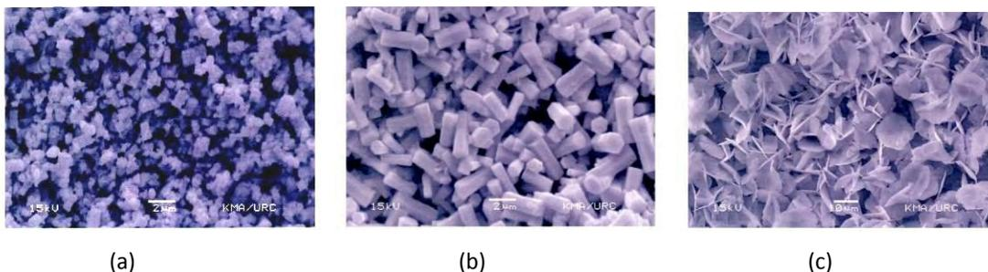
Fig. 2. SEM image of as-prepared ZnO nanorod grown on glass substrate with different solution concentration(a) 0.02M (b) 0.04M (c) 0.06M
