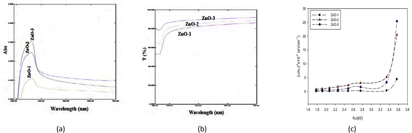
Fig. 3(a) The optical absorption spectra (b) the optical transmission spectra (c) the plot of  $(\alpha h\nu)^2$  vs  $h\nu$  for ZnO Films
