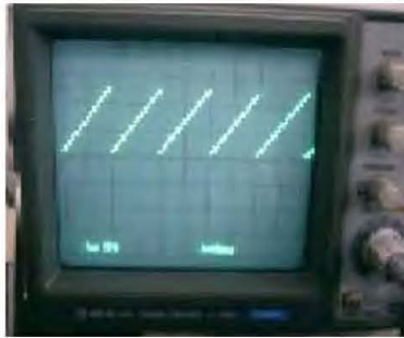
Fig. 5 Generated Saw-tooth wave
