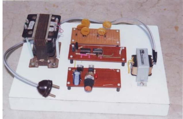
Fig. 7 Photo of constructed high voltage power supply unit
