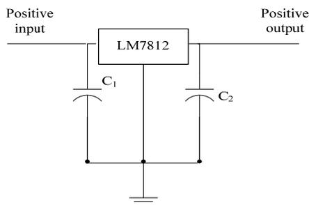
Fig. 4 Basic fixed-voltage regulator
