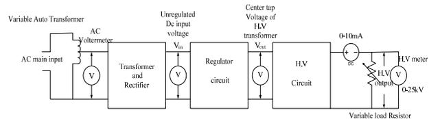
Fig. 6 A hook-up for measuring load and line regulation of H.V Unit
