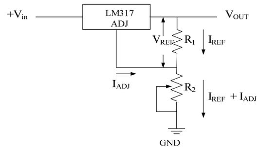
Fig. 5 Basic adjustable regulator using LM317IC
