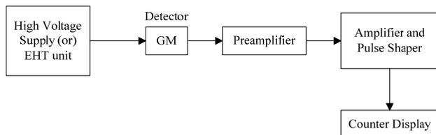
Fig. 2 Typical radiation detection system
