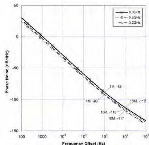
Figure 2. Phase Noise at 3.2, 5.5 and 8.0GHz
